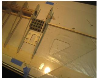
\*Position the laser cut 1/8" plywood wing servo trays one on each side of the wing center line flat on the work surface and in the notches in the # 4 ribs. Glue in place. See photo above.
