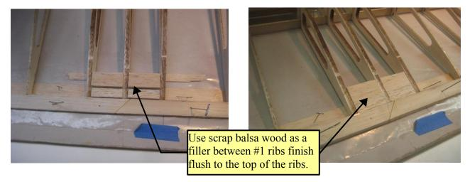
\*Make front filler support blocks using 1/4"x1/2" scrap balsa sticks cut and fit between the #1 ribs and glue behind the leading edge.
