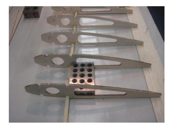
\*Place one # 4 rib each side of the wing center line spaced 3" from the previous installed # 3 rib, with its bottom notch over the bottom main spar and the rear end of the rib on the rear sheeting. Make sure the rib is 90 degrees to the work surface and the main spar. There should be a <u>no</u> gap (except for the wing servo tray notch) between the bottom of the rib and the work surface. Glue in place.
