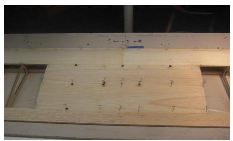
\*The wing is ready to remove from the work surface and be turned over to work on the bottom surface of the wing.
