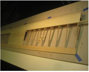
\*Trim off all the existing spars, stringers, and sheeting that may be beyond the outside surface of the last rib. Clean up any glue joints that may have excess glue that will interfere with the construction of the bottom side of the wing.
